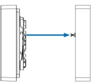
4. Hang the access point (with the mounted bracket) on the wall by aligning the key holes with the mounted screws
