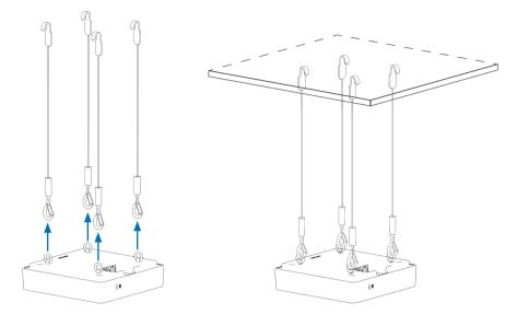
Lift the AP up, open the secure-clips, attach the hooks to the rings, and release the secure-clips to lock it
