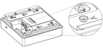
1. Place the fix-plate on the rear of the Access Point. Make sure it's positioned in the right direction as indicated.
