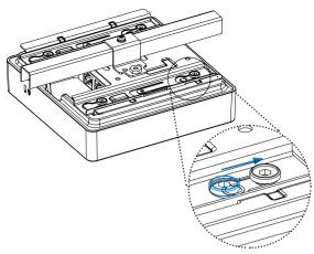
5. Align the Access Point (with fix-plate) via the key holes to the main bracket and push it to the end in the sliding-slot.
