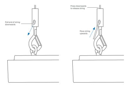
In order to adjust the height of the AP upwards, pull the end of the string further out of the wire gripper. To adjust it downwards, press the top of the wire gripper to release the wire first.
