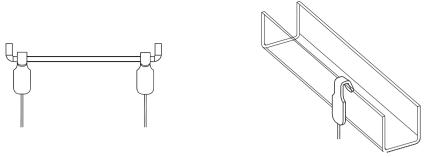
Find a suitable place on the ceiling to hang the 4 suspend-wires by using the anchor feature
