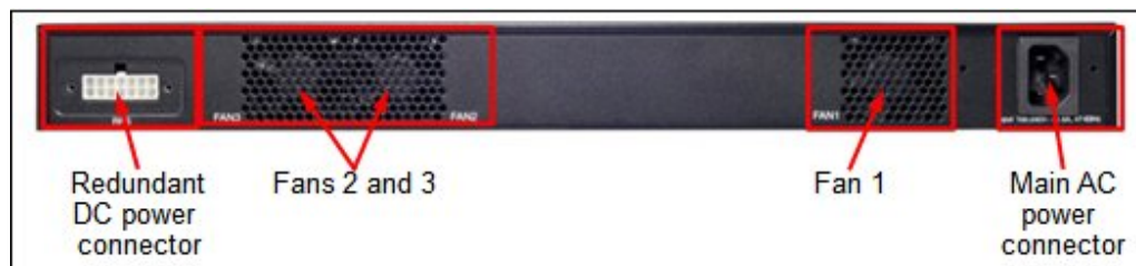
Figure 4. Rear panel of the RackSwitch G7052
